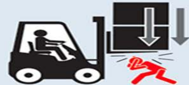
Crushed between forklift and a surface
