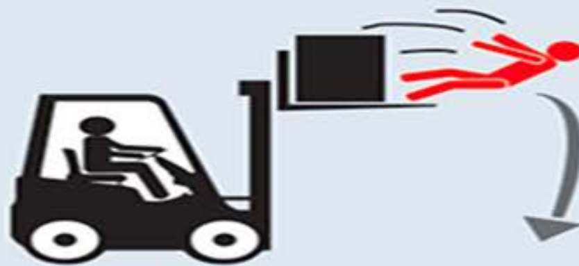
Fall from platform on the forks
