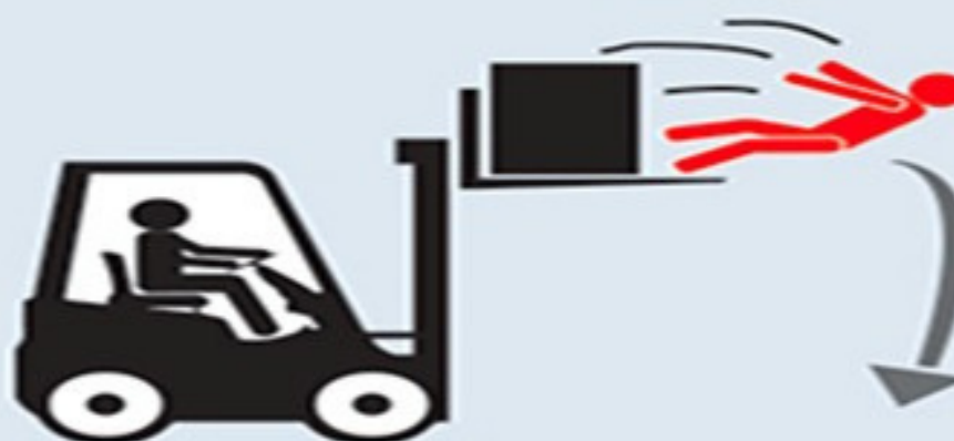
Fall from platform on the forks
